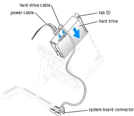
5. Connect a power cable to the drive.
