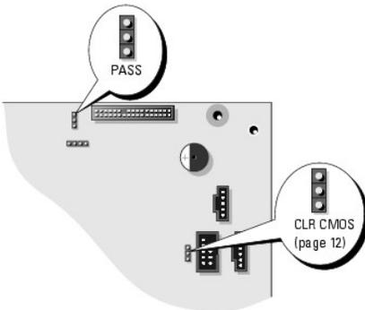
2. Locate the 3-pin password jumper (PSWD) on the [system board](#), and attach the jumper plug to pins 2 and 3 to clear the password.
