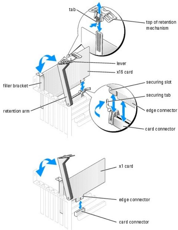
3. If you are installing a new card, remove the filler bracket to create a card-slot opening. Then continue with [step 5](#).
