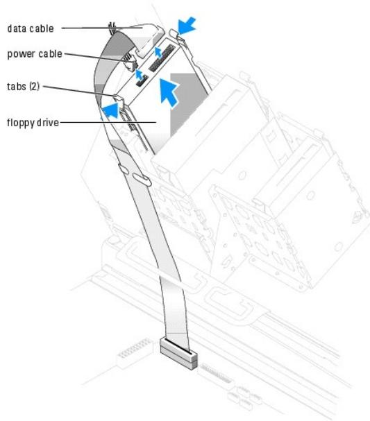
3. Press inward on the two tabs on the sides of the drive, slide the drive upward, and remove it from the floppy-drive bay.
