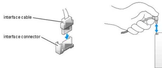
Most interface connectors are keyed for correct insertion; that is, a notch or a missing pin on one connector matches a tab or a filled-in hole on the other connector.
