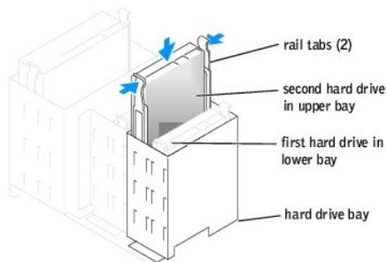
7. Connect a power cable to the drive.
