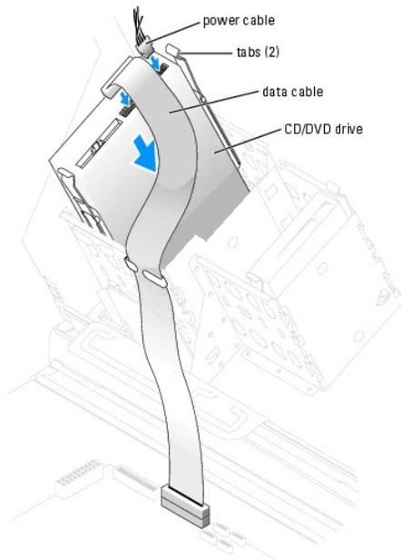
6. Check all cable connections, and fold cables out of the way to provide airflow for the fan and cooling vents.
