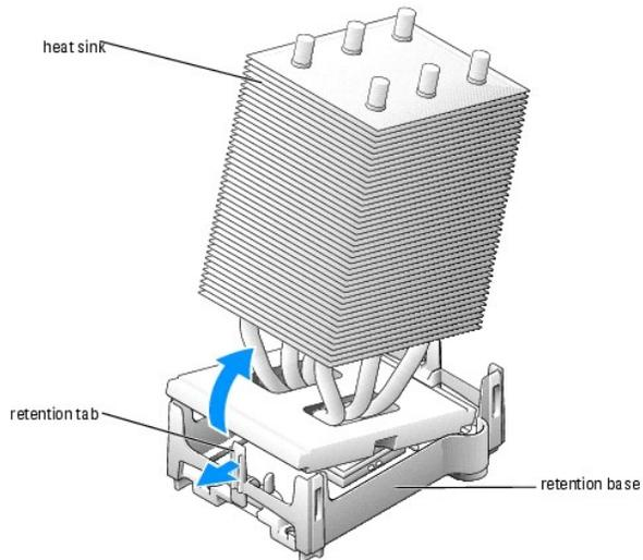
**➡ NOTICE:** If you are installing a processor upgrade kit from Dell, discard the original heat sink. If you are *not* installing a processor upgrade kit from Dell, reuse the original heat sink and blower when you install your new processor.
