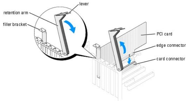
3. If you are installing a new card, remove the filler bracket to create a card-slot opening. Then continue with [step 5](#).
