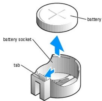
4. Insert the new battery into the socket with the side labeled "+" facing up, and snap the battery into place.
