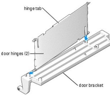
2. Attach the door bracket/door hinge assembly to the door, starting with the lower part of each door hinge.
