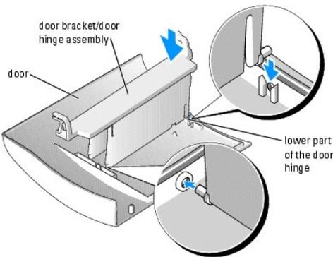
3. Attach the drive door to the computer, starting with the bottom bracket hinge.
