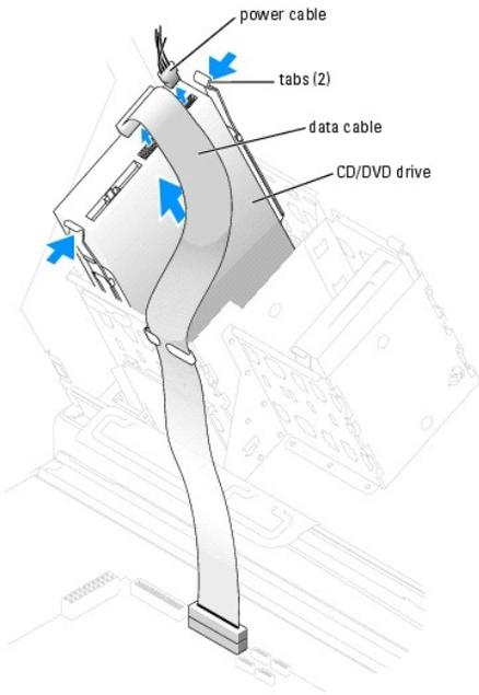
3. Press inward on the two tabs on the sides of the drive, and then slide the drive upward and remove it from the drive bay.
