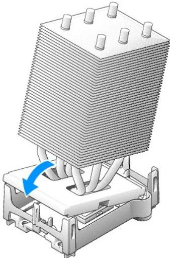
8. Reinstall the retention module clips.
