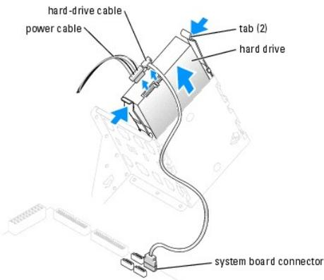
4. Press in on the tabs on each side of the drive and slide the drive up and out.
