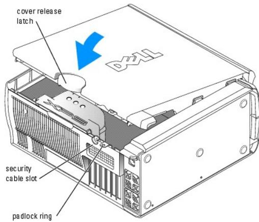
6. If you are using a padlock to secure your computer, install the padlock.
