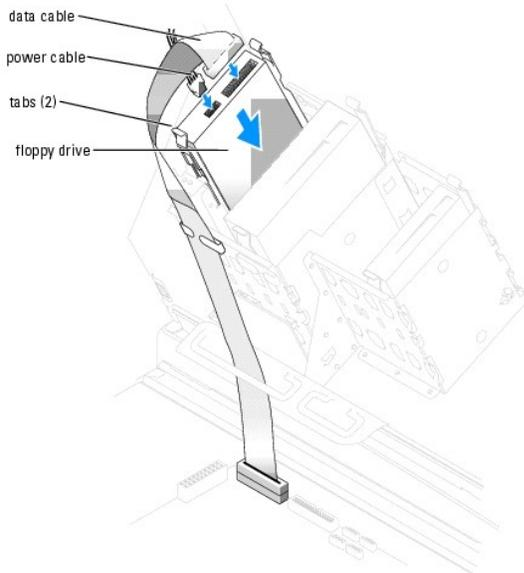
3. Attach the power and data cables to the floppy drive.
