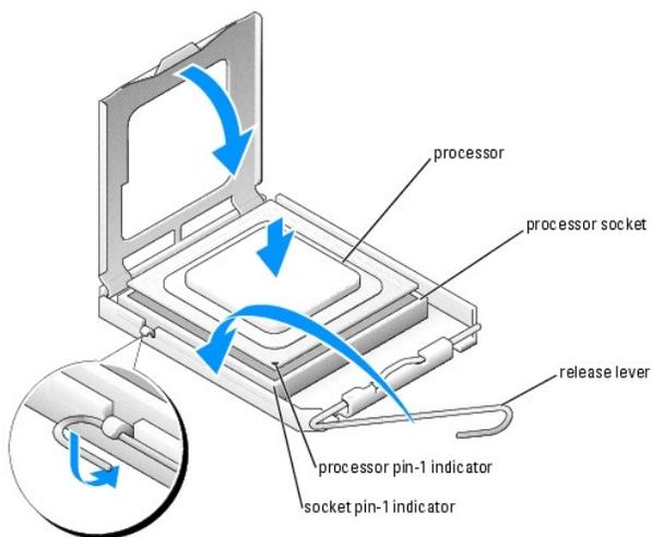
➔ **NOTICE:** Socket pins are delicate. To avoid damage, ensure that the processor is aligned properly with the socket, and do not use excessive force when you install the process. Be careful not to touch or bend the pins on the system board.
