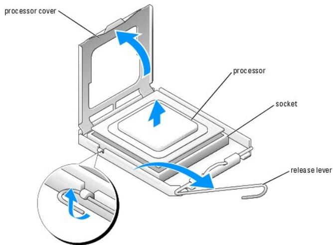
8. To remove the processor from the socket, lift the processor vertically in one motion.
