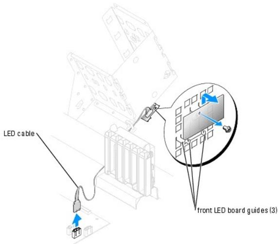
To replace the front LED board, perform the [removal procedure](#) in reverse.
