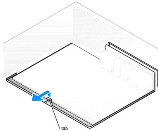
7. Pull up on the two tabs, slide the system board assembly toward the front of the computer, and then lift the assembly up and away.
